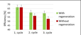
**Fig. 1**. Toluene removal efficiency obtained with  $Pt/\gamma$ -Al<sub>2</sub>O<sub>3</sub> for cycles with/without plasma regeneration.
